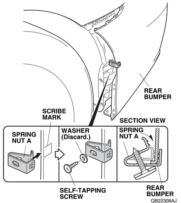
10. Remove the washer and self-tapping screw. Discard the washer, it will not be reused.
