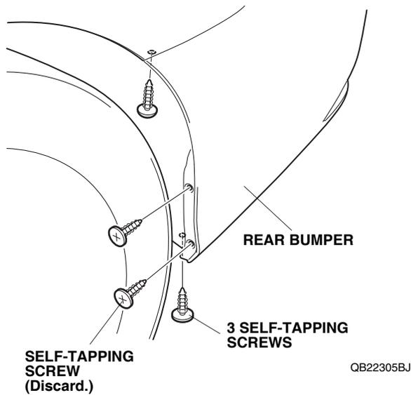
7. Pull away the rear bumper as shown. Using a pushpin, pierce the center of the scribe mark on the rear bumper.
