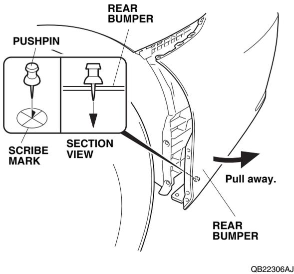
8. While wearing eye protection, drill an 8 mm hole through the pierced mark:
